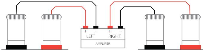
Loudspeaker cables can have a noticeable effect on sound quality. Choose a good quality cable with high purity conductors and low-loss insulation. Some Spendor loudspeakers can be bi-amped or tri-amped. Ask your retailer for advice on cables and connection options to best suit your system.
